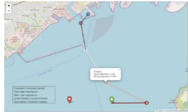
Figure 5: LIME-based highlighted trajectory. The historical trajectory is depicted and the most important parts of the historical route are highlighted based on the LIME weights.
