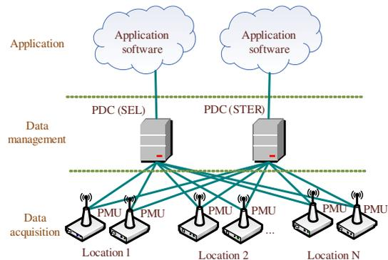
Fig. 2. Communication architecture.
