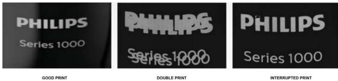
Figure 4. Samples of three types of images: (a) good (no defect), (b) double-print (defect), and (c) interrupted print (defect).
