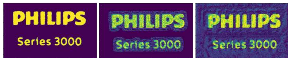
Figure 9. Original (left) vs. FGD (middle) and PGD (right) attacks— Dataset_2 . FGD attack is slight, while PGD adds a significant amount of noise and color alteration.
